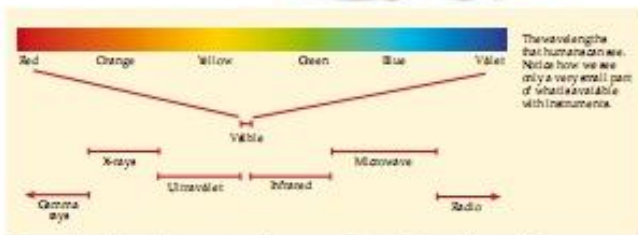
Electromagnetic wavelengths – those we can see, and those we can only detect using instruments (see page 44).
